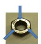
Picture 9 Install nut crimp end facing down
